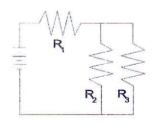
Questions 6 and 7 refer to the following: The diagram to the right represents an electric circuit consisting of four resistors and a 12-volt battery.
